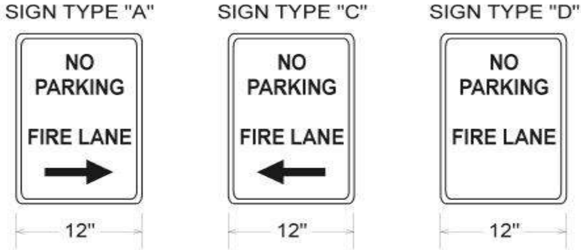
FIGURE D103.6 FIRE LANE SIGNS
